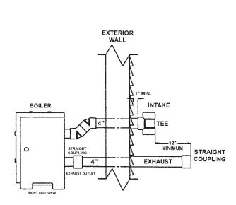
\*\*IMPORTANT NOTE: All vent pipes must be glued, properly supported and the exhaust must be pitched a minimum of a 1/4" per foot back to the heater (to allow drainage of condensate).
